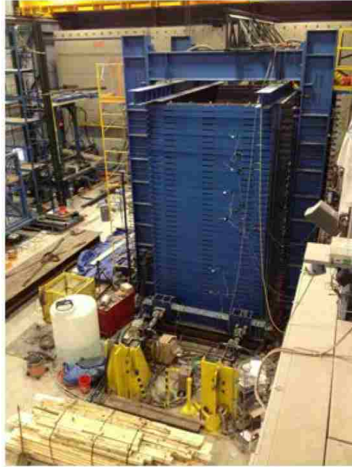
Figure 3-2: Actuators Placed against the Laminar Shear Boxes
